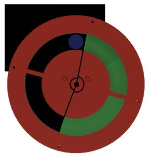
Part "a" is the hub attached to the motor shaft. Part "b" is a combination of 2 or more parts that can slide inside the other and this combination sits in the cavity of "a". Part "c" covers the hub "a" with a 360-degree scale over it. Part "d" sits inside the cavity of "c" without making any contact and is fixed with the hair dryer holder. Further a pipe is connected to part "d".
